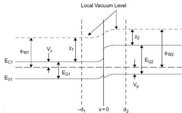
Fig. 2 Energy band model of a heterojunction interface
