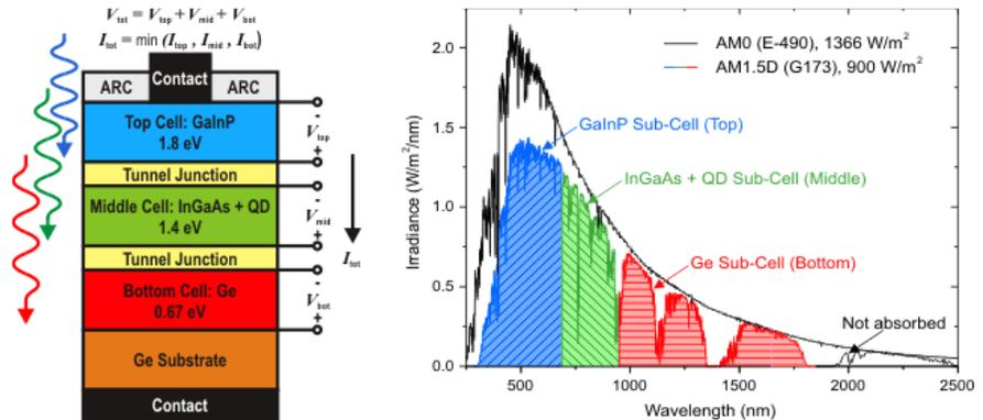
Figure 1 A high-efficiency multi-junction solar cell's epitaxial design and absorption spectra[1]
